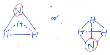
This is the basis of the MASER (Microwave Amplification by Stimulated Emission of Radiation - the precursor of the LASER).
