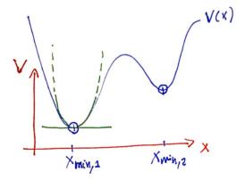
It is natural for the particle to come to rest near one of the potential energy minima,  $x = x_{\min,1}$  or  $x_{\min,2}$ . Small perturbations will let the particle explore the potential energy landscape near the minimum  $x = x_{\min}$ . To describe such motion one can carry out a Taylor expansion,
