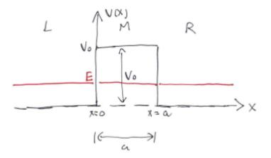
Classically, particle cannot get through barrier. Let us see what happens in quantum mechanics. Let us obtain the stationary states  $|E(0)\rangle$  i.e. solutions to the time-independent Schrödinger equation. We can then obtain the probability current density j(x) using Eq. (6.24).
