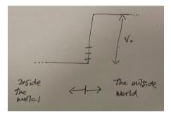
However, unlike classical particles, electrons can overcome this barrier, even when their energy is lower than the barrier itself. This is called **quantum-mechanical** "tunnelling" and it has been verified extensively. Indeed, it forms the basis of the **Scanning Tunnelling Microscope** (STM), an experimental technique that we have mentioned before in this course.
